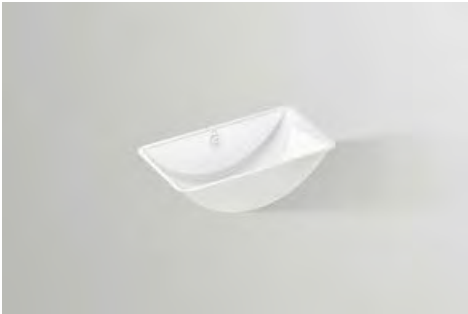
Undermount basin, rectangular, l/w/h 507/273/143 mm, glazed steel, without tap hole, with overflow, included fixing set, overflow set
