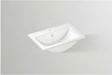
Built-in basin, rectangular, l/w/h 585/405/143 mm, glazed steel, with one tap hole, with overflow, included fixing set, overflow set
