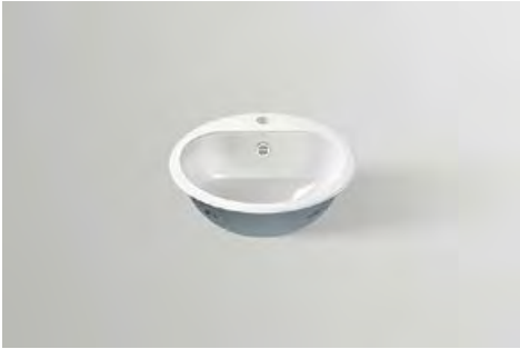
Built-in basin, round, l/w/h 475/475/186 mm, glazed steel, with one tap hole, with overflow, included fixing set, overflow set, PVC seal
