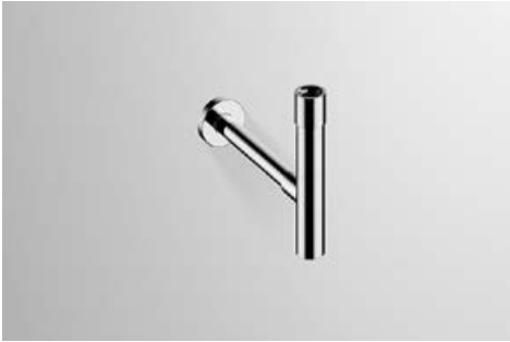
Bottle trap, l/w/h 45/370/297 mm, chrome-plated, 1 1/4" connection thread, immersion tube, adjustable in height from 135 to 205 mm, adjustable depth from 90 to 370 mm
