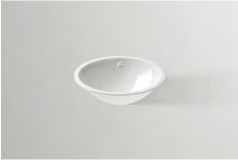
Built-in basin, oval, l/w/h 525/425/150 mm, glazed steel, without tap hole, with overflow, included fixing set, overflow set
