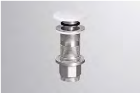
Drain valve, round, l/w/h 74/74/120 mm, Ø 1 1/4", with open/closed function, this basin requires an overflow, valve cap, white glazed
