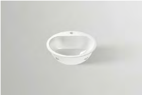
Built-in basin, round, l/w/h 475/475/186 mm, glazed steel, with one tap hole, without overflow, included fixing set
