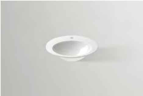
Built-in basin, oval, l/w/h 500/400/110.5 mm, glazed steel, with one tap hole, without overflow, included fixing set
