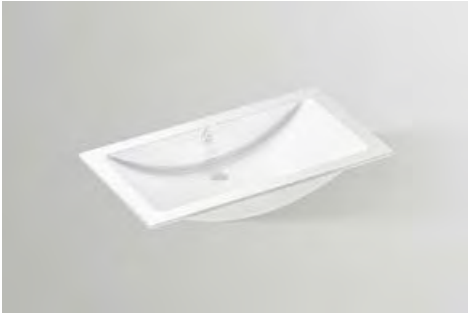
Built-in basin, rectangular, l/w/h 800/450/120 mm, glazed steel, without tap hole, with overflow, included fixing set, overflow set
