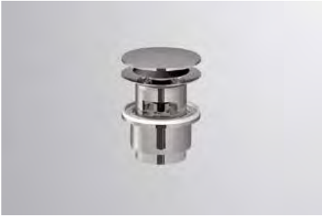
Drain valve, round, l/w/h 63/63/74 mm, Ø 1 1/4", with open/closed function, this basin requires an overflow, valve cap, chrome-plated
