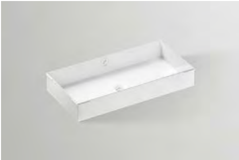
Undermount basin, rectangular, l/w/h 744/369/111 mm, glazed steel, without tap hole, with overflow, included fixing set, overflow set, optimised for installation directly under the laminate layer of a coated counter top
