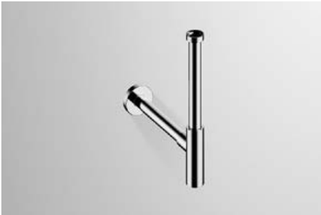
Bottle trap, l/w/h 45/390/419.5 mm, 1 1/4" connection thread, immersion tube, adjustable in height from 75 to 330 mm, adjustable depth from 90 to 390 mm
